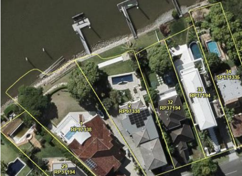
Figure 2(c): ‘Adjutments (disparity between adjoining boundaries)’ between surveys completed at differing temporal events, Brisbane River, Qld (Source: Queensland Globe)
