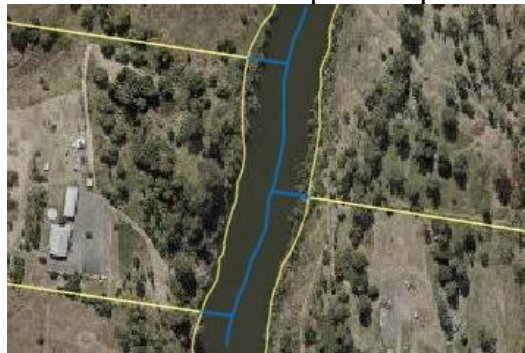
Figure 1: Sample of Cadastral watercourse boundaries (Contiguous Single line watercourse in blue and Two-line non-contiguous watercourse in yellow) (Source: Queensland Globe)
