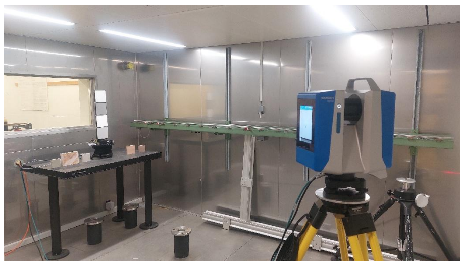
Figure 1: Experimental setup in the climate chamber, with the targets on the table (left) measured by the Z+F Imager 5016 (right).
