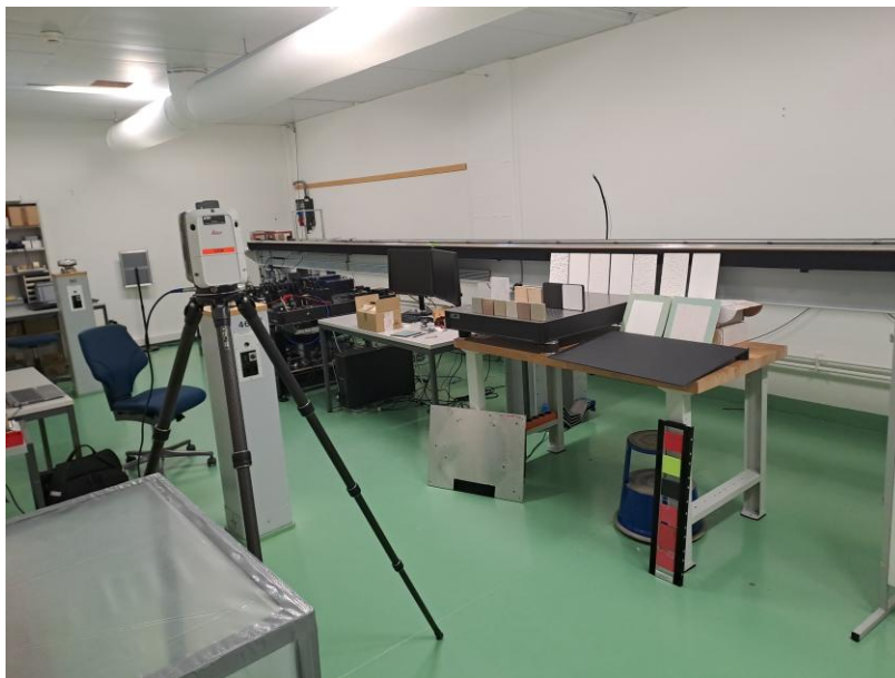
Figure 2: Experimental setup in measurement laboratory, with the targets on the table (right) measured by the Leica RTC360 (left).
