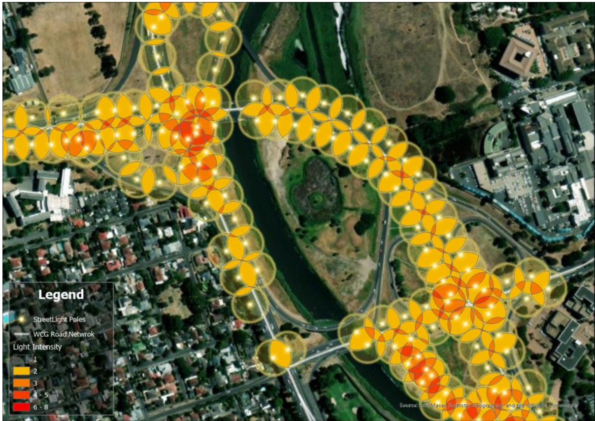
Figure 5: Buffer analysis revealing light coverage and derived intensity polygons within a major interchange.
