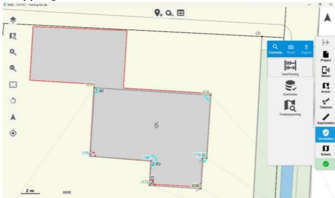
Figure 2: Measuring a building in Delfy. Note the green checkmark in the bottom right of the menu indicating all checks are successful at the moment
