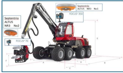
Fig. 2.04 Forestry vehicle 3D mapping : Komatsu harvester - GNSS-TLS
