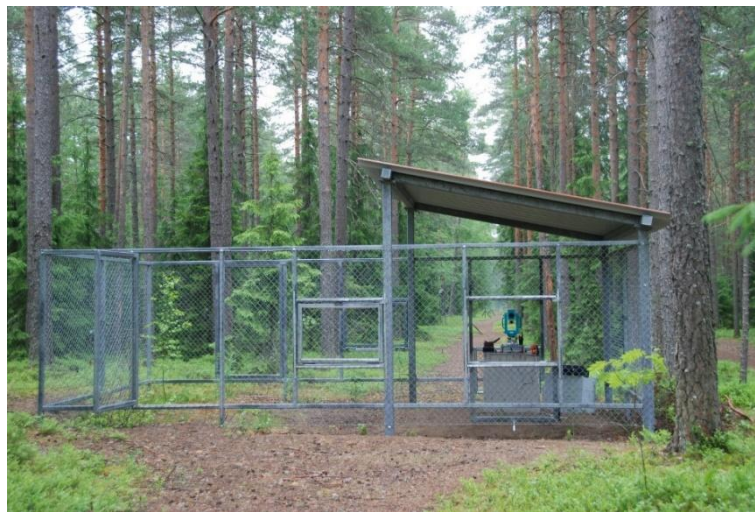
Figure 3. For EDM calibrations, Nummela Standard Baseline has six observation pillars with centring plates at 0, 24, 72, 216, 432 and 864 metres. The actual baseline (with the known lengths from the interference measurements) is preserved between the six underground markers two metres apart from the observation pillar line. The connection between the two lines is annually checked with the theodolite-based projection measurements with up to 0.2 mm standard uncertainty. Photo: J. Jokela, FGI.
