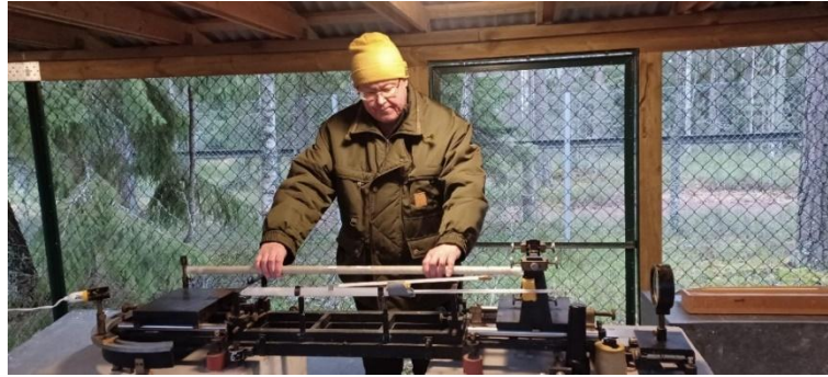
Figure 2. After two months of arduous but successful measurements Jorma Jokela is removing the quartz metre no. VIII from the Väisälä interference comparator at the Nummela Standard Baseline in December 2024. Photo: T. Saari, FGI.
