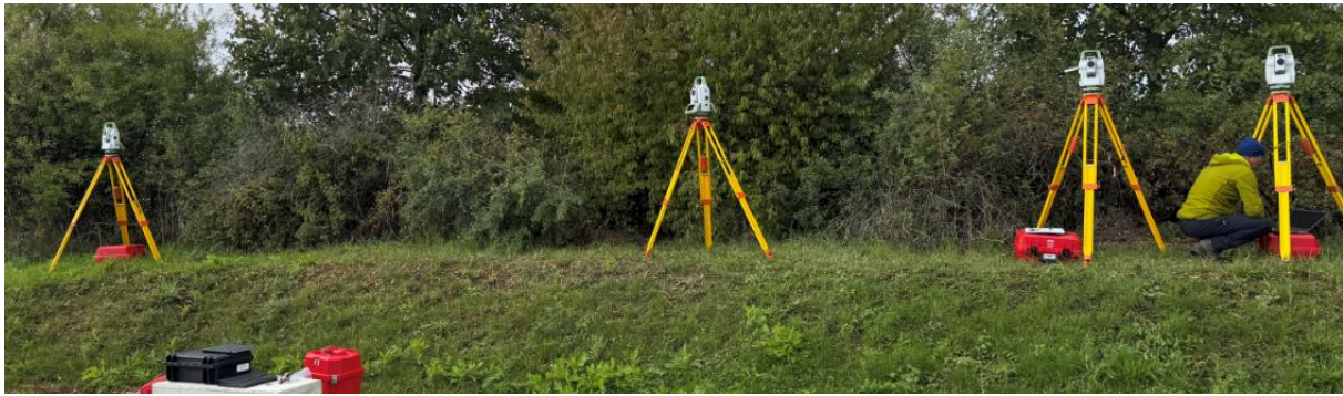
Control measurements: classical displacement monitoring – four measurement points requiring four total stations (Bautzen)
