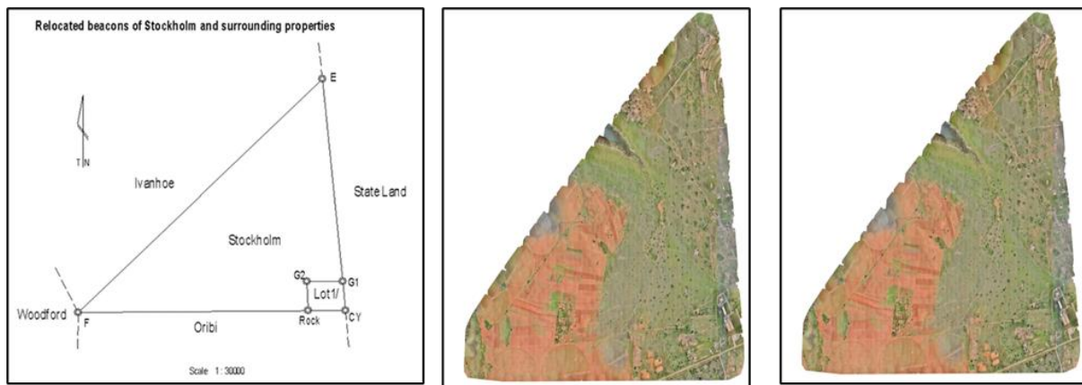
(a) (b) (c) Figure 4: a) Stockholm beacons, b) Othomosaic from 20 GCPs, c) othomosaic from 6 GCPs
